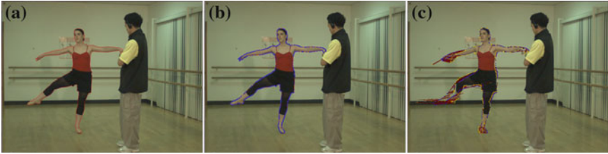
Fig. 2 Creation of feature points and calculation of optical flow from object contour. a Object extracted from the n th frame by the operator, b Feature points created from the object contour in (a) , c Results of tracking feature points of (b) along optical flow in the n + 1 th frame
