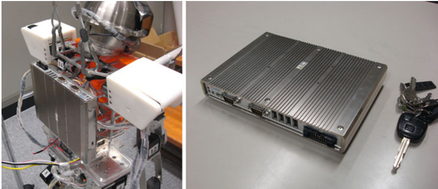
Fig. 2 ETC-A013 computer mounted in biped robot
