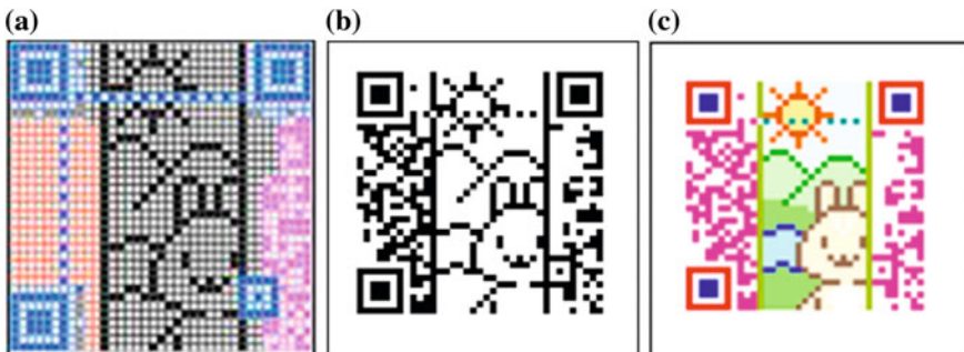
Fig. 10 Typical example of colored two-dimensional code. a Dotted image is inserted, b two-dimensional code, c color conversion
