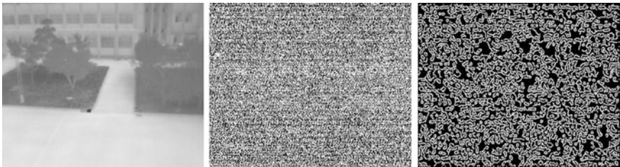
Fig. 4 An example of no moving object case. Left Input image. Middle Mahalanobis distance map. Right Canny edge detection results
