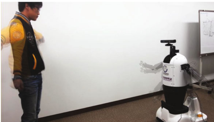
Fig. 8 Test using humanoid robot dual arms
