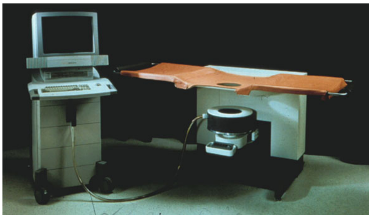
Fig. 15.9 Clinical DT prototype scanning system with annular array mounted on a vertical translation stage below a modified breast biopsy table. From André et al. (1997)
