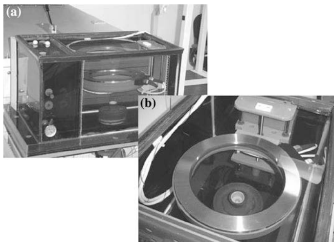
Fig. 15.7 Ring transducer array in the water tank that is positioned below the patient table for scanning. From Duric et al. (2005)
