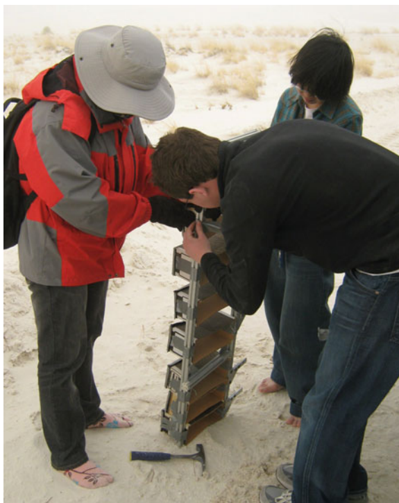
Fig. 3 Constructing the traps for sand collection (Photo of White Sands, New Mexico Earth Surface Processes field class, 2011)
