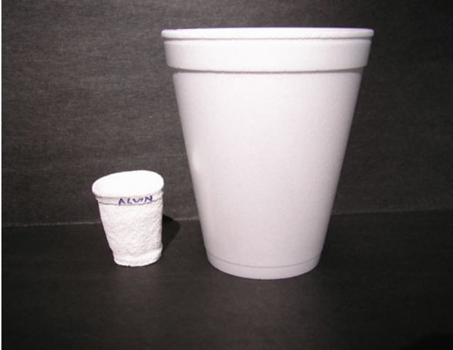
Fig. 4 A 16-oz. milkshake cup ( right ) next to the same type of cup taken down to a depth of over 3,000 m outside of the submersible ALVIN, illustrating the great pressures at depth in a way that was very tangible to students
