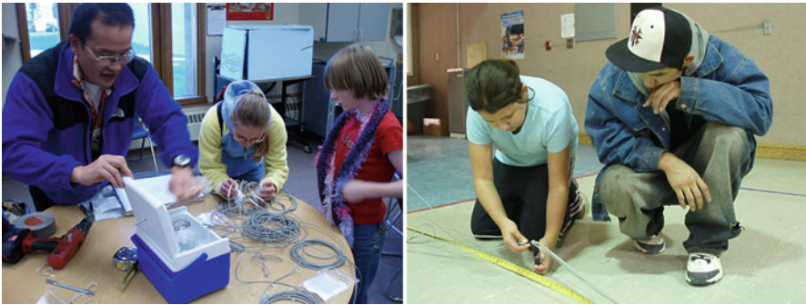
Fig. 3 Students prepare ice bath for calibration process ( left ) and set up sensor length for different depths ( right )
