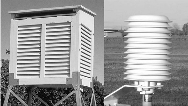
Fig. 20.2 A standard Stevenson Screen ( left ) and a Gill radiation shield ( right )
