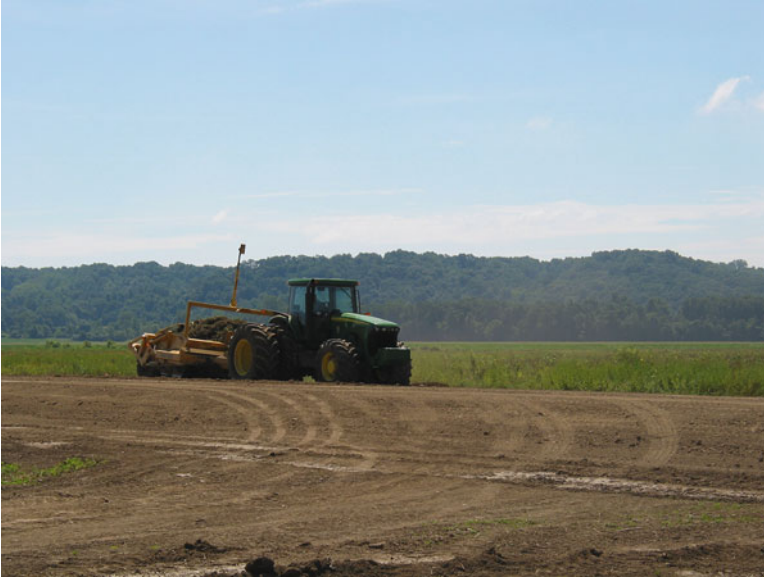
Fig. 3.9 Photograph of modern earth moving machinery using tractors and dirt pans
