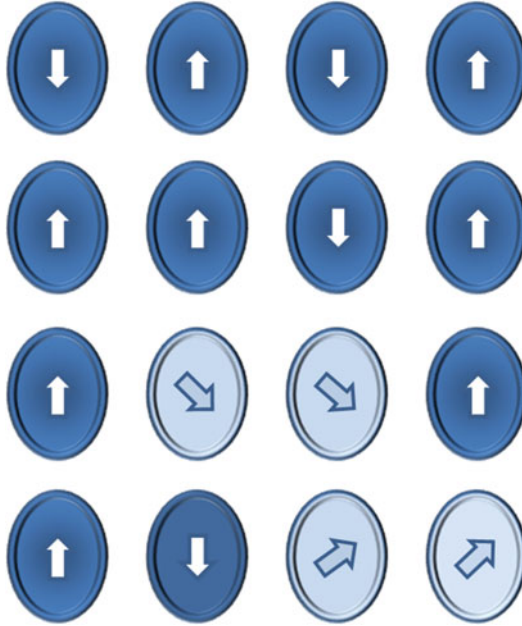
Fig. 15 Bennett clocking scheme for propagating a binary logic bit unidirectionally along a chain of nanomagnets or logic wire. ( First row ): A chain of magnets in the ground state. Dipole interaction ensures the anti-ferromagnetic ordering. ( Second row ): Magnetization of the first magnet is flipped with an external agent, but the second magnet does not necessarily respond since the dipole interactions from its left and right neighbors are equal and opposite, resulting in no net dipole interaction. ( Third row ): The second and third magnets are stressed to rotate the magnetization. The second magnet is freed from stress and it flips since the dipole interaction from its left neighbor is now stronger than that from its right neighbor. At the same time, the fourth magnet is stressed. At the end of this cycle, the input bit has propagated through the first magnet on the right. By repeating this cycle, the bit can be progressively propagated to the right unidirectionally
