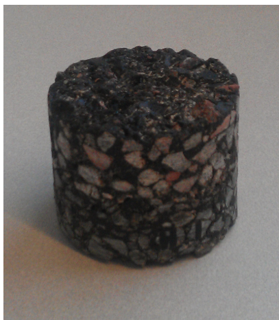
Fig. 2 Porous asphalt concrete sample used in the present study
