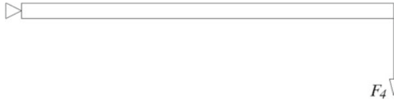
Fig. 3.7 This bar is articulated around its left extremity. A vertical force ( F_4 ) is applied on the right extremity. This unstretched bar displays a zero stiffness along the vertical
