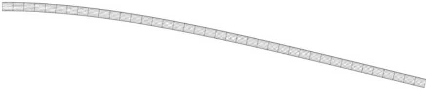
Fig. 7.10 Vertical deflection of a beam calculated with the model. The beam is fixed on the left and free to bend on its own weight on the right . The conditions are the same as in the text except for the bending rigidity, which is ( EI = 16.493 \text{ N.m}^2 ), ten times less than the case of Table 7.3 and Fig. 7.11 to highlight the deformation
