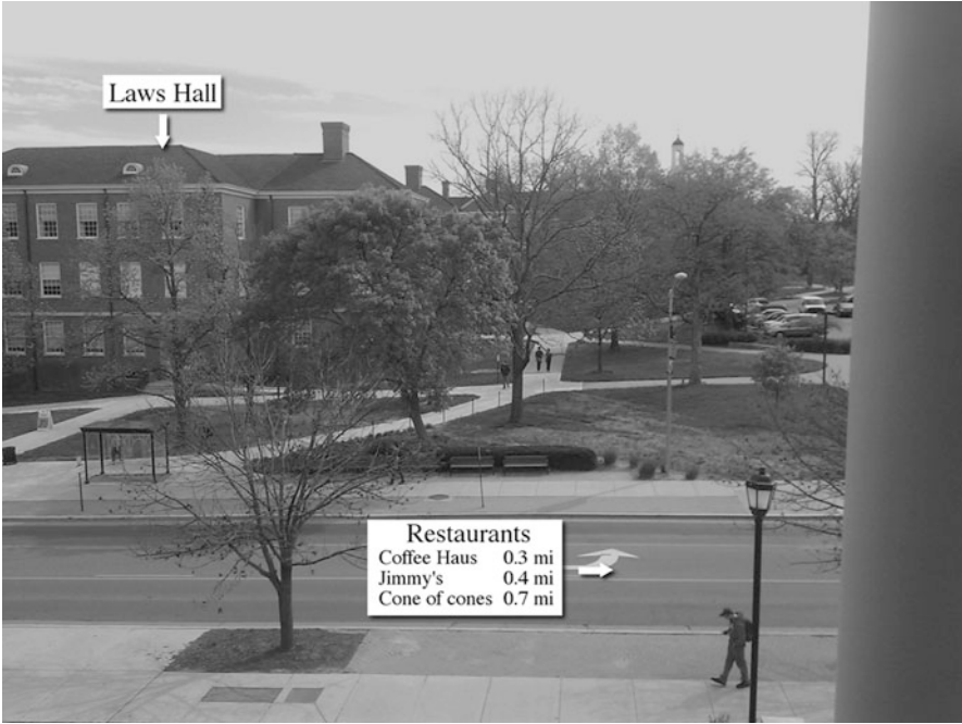
Fig. 8.4 A simulated view of an augmented reality browser for a smart-phone. The user looks at the screen of the smart-phone, and sees helpful information overlaid on the world, including the names of landmarks and directions to food and lodging
