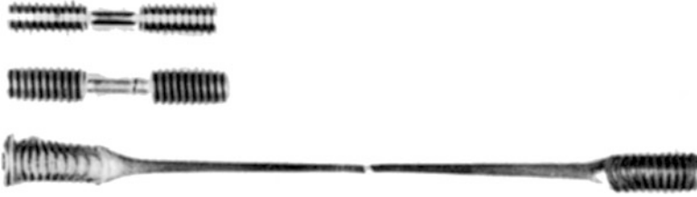
Fig. 1 Steel test specimen repeatedly temperature cycles through a phase change. From Greenwood [5]
