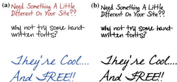
Fig. 20.2 a Example image of a handwritten text document with multiple pen intensities. b Binarization output using proposed adaptive approach
