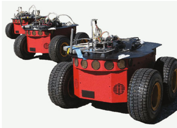
Fig. 7.7 Pioneer robots from Adept Mobilerobots LLC., with GPS receivers, digital compass and wireless communication units
