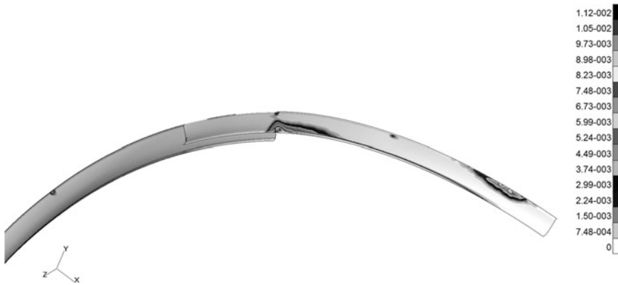
Fig. 43.11 Map of plastic strain of part of arch yielding support under dynamic load
