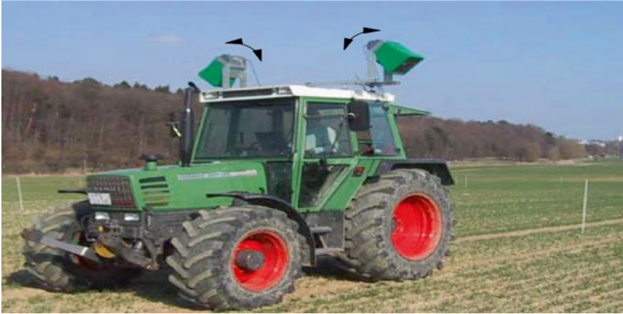
Fig. 9.31 Simultaneous sensing of the fluorescence ratio (F680/F735) and of estimates of the plant density per unit area. The plant density is sensed by the number of signals per unit of area above a noise level. The inclination of both sensors perpendicular to the direction of travel oscillates with a frequency of 1–2 Hz while driving through the field. Hence the field surface is scanned for signals (From Thoren 2007, supplemented)
