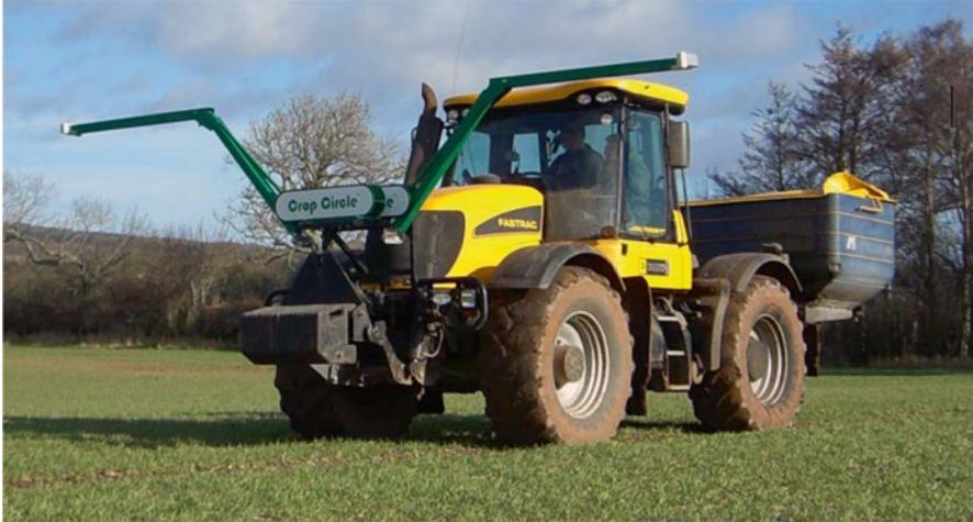
Fig. 9.24 Control of nitrogen spreading via reflectance sensing based on artificial light with vertical viewing of the canopy from transverse booms in front of the tractor (Crop Circle concept, photo from Wilson J., SoilEssentials Ltd., England)
