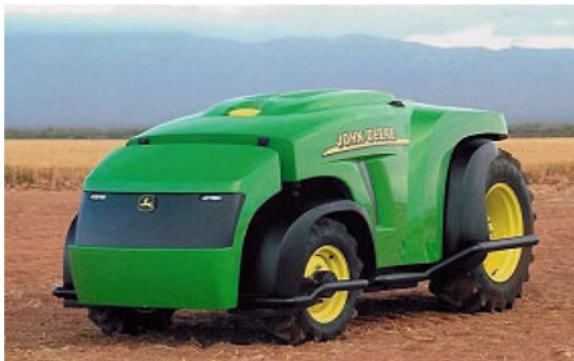
Fig. 7.15 Unmanned tractor (Courtesy John Deere Co.)
