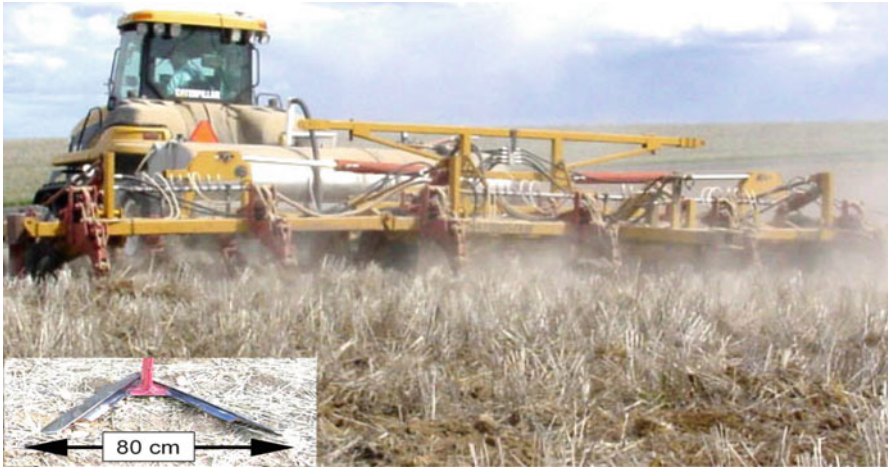
Fig. 7.13 Setting a moisture line in a fallow field by an under-cutter. The insert shows the main tool. The soil surface is covered with anchored crop residues (Photo from Schillinger, altered)
