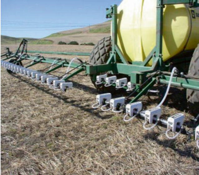
Fig. 6.5 Sprayer boom with optical sensors for spot spraying of weeds in a fallow field (Courtesy of Trimble Agric. Div., Westminster, USA, altered)
