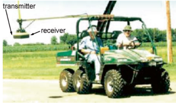
Fig. 5.19 Sensing surface reflectance of ground penetrating radar (From Redman et al. 2003, altered)
