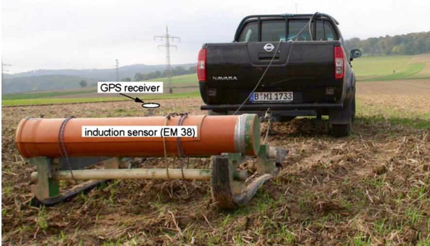
Fig. 5.4 Online and on-the-go sensing of soil electrical conductivity by electromagnetic induction. The sensing instrument (EM 38 of Geonics LTD, Canada) can be moved on a sled, on a cart or even be carried by hand. In order to prevent interference from metal, some distance to the vehicle is needed (Photo from Agri Con GmbH, Jahna, Germany, altered)
