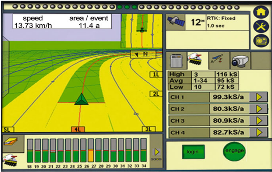
Fig. 4.5 Display of an user interface to an automatic guidance system. The lightbar ( top ) indicates cross-track errors. The signals from two different GNSS satellite systems can be used simultaneously in order to improve availability. Site-specific section control of implements ( e.g. sprayer) is possible (Courtesy of Trimble Agric. Div., Westminster, USA, altered)
