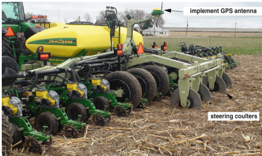
Fig. 4.11 Active guidance of a seeding machine on a side-slope. The GPS antenna on the roof of the tractor is hidden (From Orthman Mfg.Co., altered)
