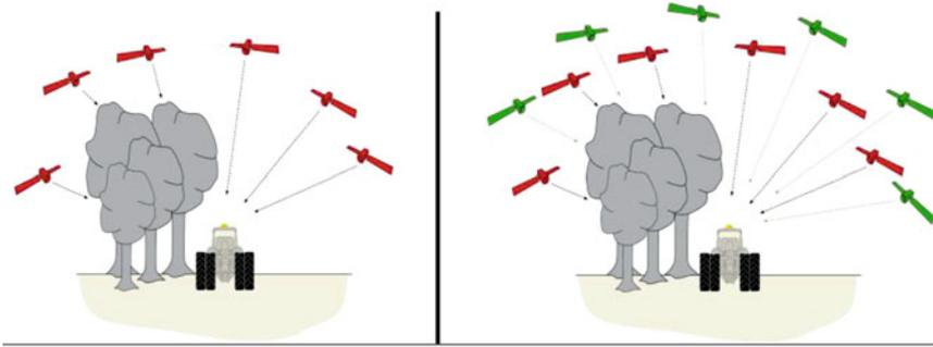
**Fig. 3.9** The position of the receiver on the tractor is the same in both drawings. In the *left* drawing, the signals from only three satellites get to the receiver, which in most cases is not sufficient for georeferencing. In the *right* drawing – because of more satellites – georeferencing is possible (From graphs by Poloni 2009)
