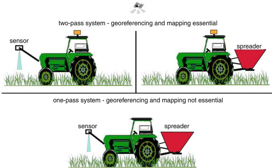
**Fig. 3.7** Tractor-based control for site-specific spreading of fertilizer with or without mapping
