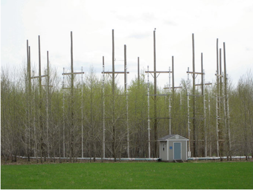
Fig. 6.2 One of twelve experimental plots at the Aspen Free Air CO 2 Enrichment (FACE) facility in northern Wisconsin, United States. Trees were exposed to combinations of ambient and elevated carbon dioxide and ozone in order to study their effects on various physiological and ecological processes, including their interactions with key herbivores
