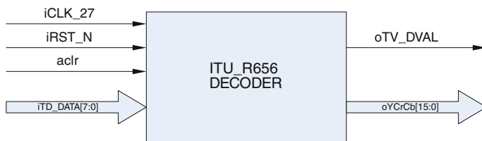
Fig. 5 ITU-R656 decoder block connection
