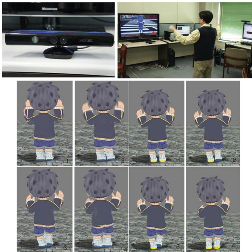
Fig. 2 Top left: Kinect sensor for experiments. Top right: An 3D character is controlled by the user in on-line puppetry manner. Bottom left: Screen shots before applying foot skating cleanup. Bottom right: Screen shots after applying foot skating cleanup. Yellow ball indicates whether this frame is constrained or not
