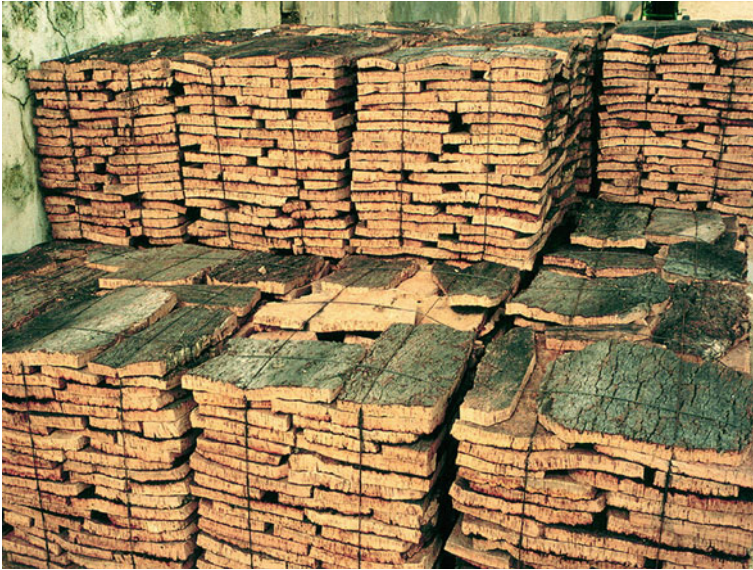
Fig. 2.15 Slabs of cork, steamed and pressed flat, await transport and conversion into cork bottle stoppers, flooring, or other uses. Once considered an essential strategic product, and used as an insulator and as a flexible gasket-sealant, cork remains a high-value product of the dehesa (and the Portuguese montado ), but faces competition from the plastic “stopper” industry in wine-producing countries that are not able to produce cork and must buy their supply. (Photograph by P. F. Starrs)
