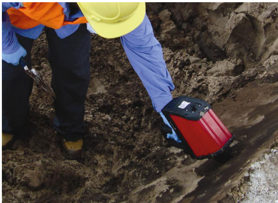
Fig. 3.10 ExoScan 4100 during field use in a soil sampling pit (Photo courtesy Agilent Technologies)
