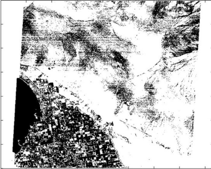
Fig. 13.2 Graybody-pixel map for the Salton Sea (black = gray, white = bare). A first guess graybody-pixel map was first estimated by thresholding ASTER reflectance indices to identify vegetated and water/snow pixels (e.g., NDVI), and then refined using the Thermal Log Residual (TLR) method described in the text
