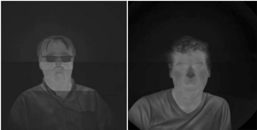
Fig. 5.13 Two images taken with the HyTES 1\text{ K} \times 1\text{ K} QWIP array, the first author is on the left . The images show that most pixels appear to be active. There's very little "dead" pixels. The image on the left uses a single point correction and the image on the right uses a two point correction. A single point correction typically takes out any offset present in the system while the 2-point correction typically removes bias and gain. There's an obvious improvement in terms of image uniformity between the two images
