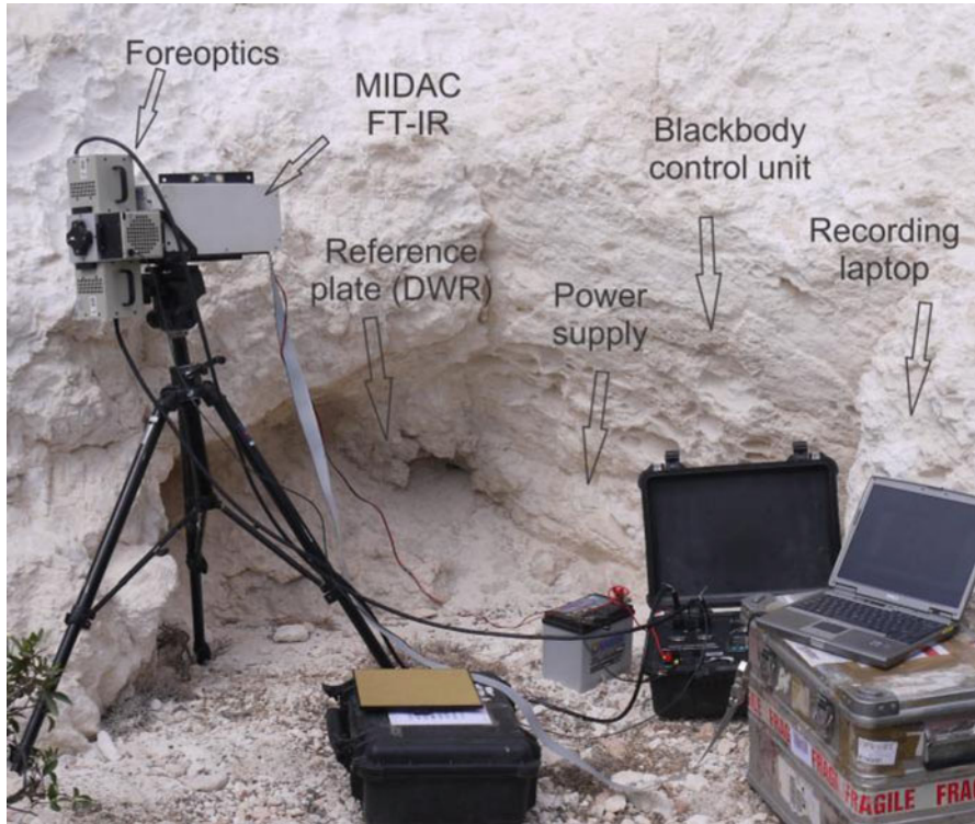
Fig. 3.7 MIDAC Illuminator at a vertical outcrop with blackbody control unit, laptop and battery (Photo courtesy Chris MacLellan, NERC-FSF)
