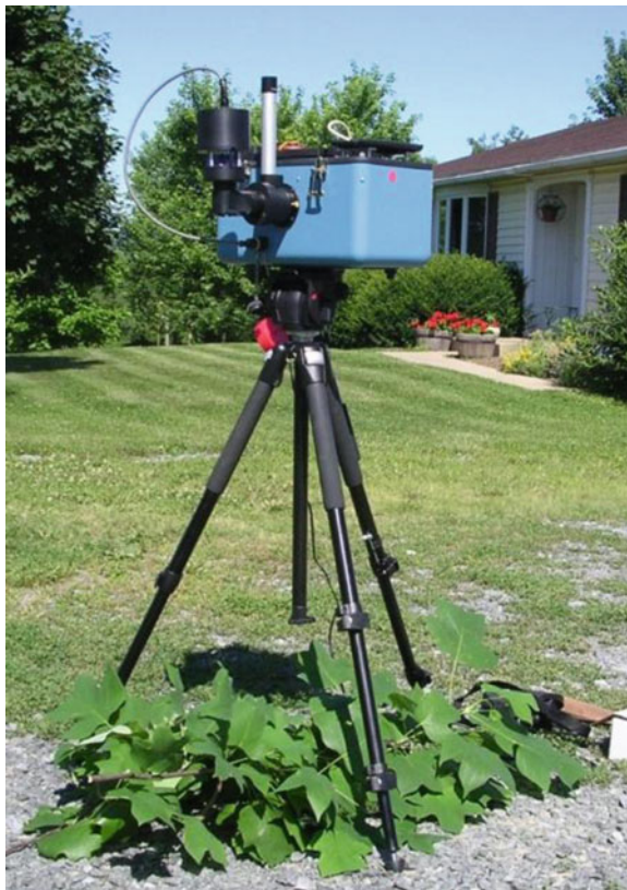
Fig. 3.6 DnP 102F \mu FTIR field spectrometer measuring vegetation detached from the canopy. The black barrel at the end of the gray power cord is the single calibration blackbody
