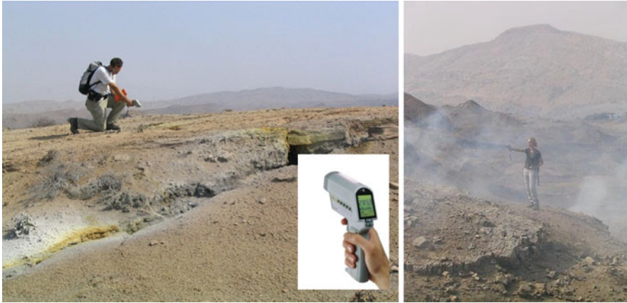
Fig. 21.4 Measuring underground coal fire related temperatures in-situ with handheld Raytek radiometers (Small image courtesy of Raytek. Photographs: C. Kuenzer ( left ), C. Hecker ( right ))
