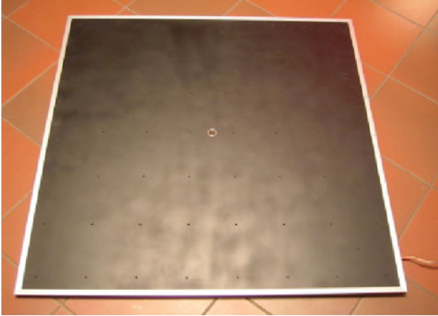
Fig. 2.2 Plane test field with active lamps (size: 1 m × 1 m)
