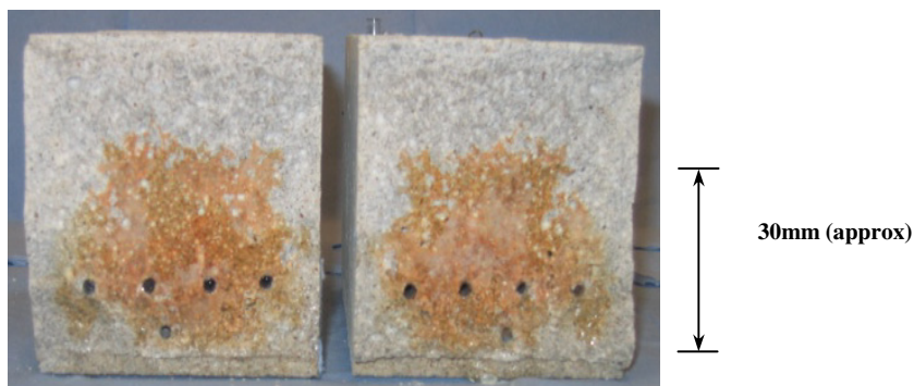
Fig.4.54 Typical glue migration and effective zone of healing for self-healed beams
