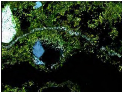
Fig. 2.10 Microphotograph showing a crack in 19th century lime mortar, filled completely by calcite (View 0.7 x 0.45 mm, cross polarized light) (a) Microphotograph showing a crack in 19th century lime mortar, filled completely by fine grained portlandite (View 0.7 x 0.45 mm, cross polarized light) (b) [2.15]
