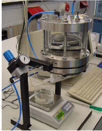
Fig. 2.20 Set-up for high pressure permeability measurements
