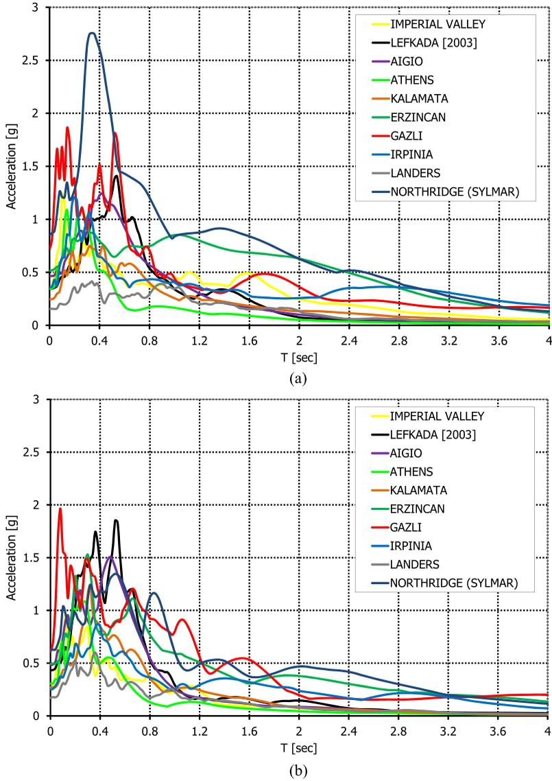
**Fig. 4** Acceleration response spectra for 5 % damping of the horizontal components of the base motions that were applied in (a) the longitudinal direction and (b) the transverse direction of the structure
