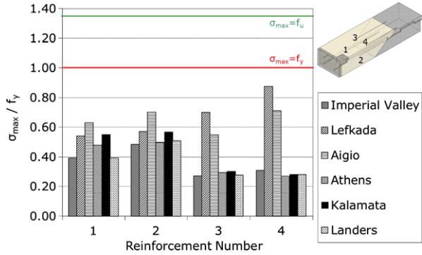
**Fig. 8** Efficiency factors of the four titanium bars used for the complement of the third drum of column 1 of the colonnade in Kos for the five earthquake excitations that do not cause collapse of the monument
