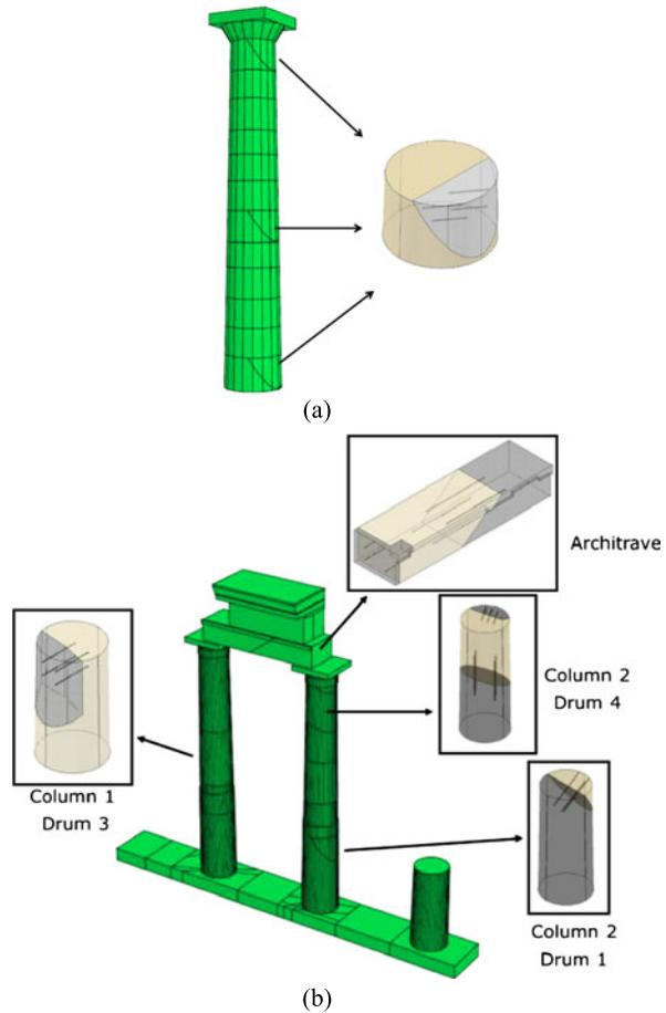
sliding can occur before these connectors are activated, since a gap of 1 to 2 cm, not filled with mortar, is commonly left between them and the edge of the mortises. Both assumptions are to the safety side and lead to the upper limit of the forces that can be induced to the reinforcement.
