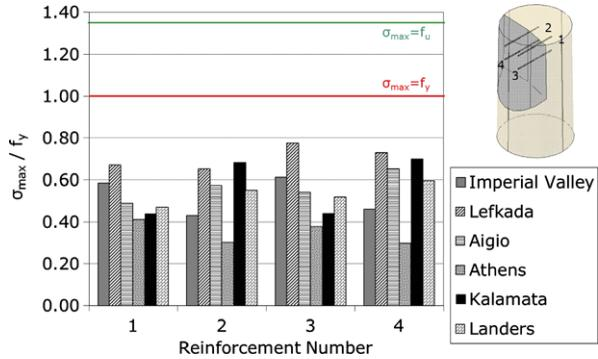
**Fig. 9** Efficiency factors of the three titanium bars used for the complement of the first drum of column 2 of the colonnade in Kos for the five earthquake excitations that do not cause collapse of the monument
