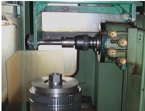
Fig. 1 Machining center modified for fly tool test
