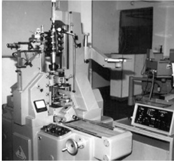
Fig. 14 Hob inspection on the device PWF 250—Klingelnberg
