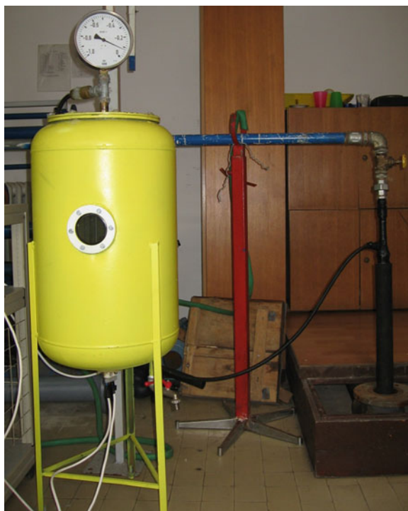
Fig. 5 Student team CFS prototype 2006/2007 (device for drinking water sterilisation)
