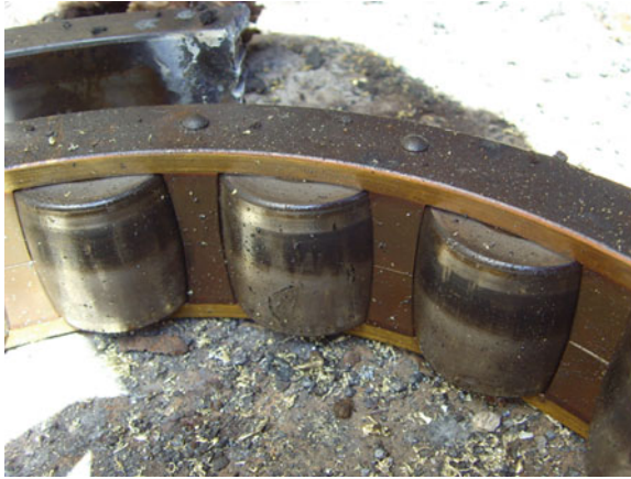
Fig. 7 The damage on the cylinder SKF NU244MA after repairing
