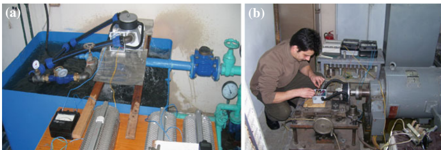
Fig. 2 Establishment of the turbine (a) and generator (b) parameters on testing rigs
