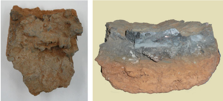
Fig. 3 On the left the uneven, partially vitrified inner surface of a piece of the rear wall of the furnace is shown. The piece is about 16 cm high and 13 cm wide and reaches from the middle to the lower end of the rear wall. From its upper rim about 3 cm were cut off, yielding samples 612/4, 612/5 and 612/6 (cf. Fig. 2). On the right, a view of the cut face of the piece left after removing these samples is shown. The piece reaches about 50 mm deep into the soil. The bright spot in the middle about 5 mm below the surface is a rather large metallic copper inclusion
