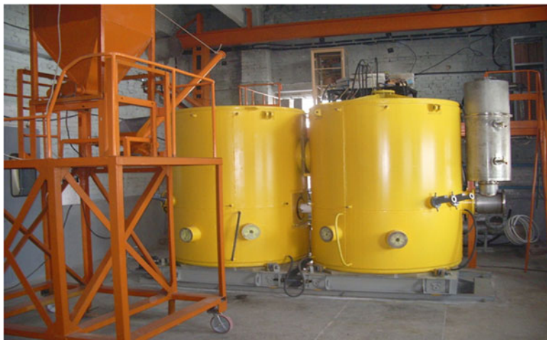
Fig. 31.8 The installation of the plasma chemical reactor of new construction for destruction of wastes (plasma torch power-500 kW; gas flow rate –50–150 kg/h; waste capacity up to 200 kg/h)
