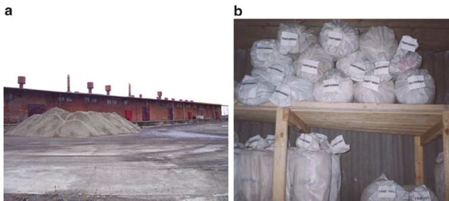
Fig. 31.2 Improvement of obsolete pesticides storage conditions: (a) initial storage conditions; (b) after repacking and labeling of obsolete pesticides
