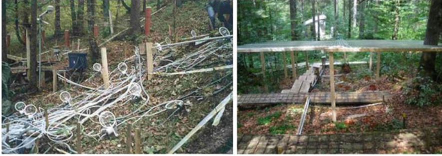
Fig. 6.4 Automated chambers for the measurement of the soil carbon dioxide ( left ) and a roof to temporarily create drought conditions in a field experiment ( right ); Experimental site: mature, spruce-dominated forest, Mühleggerköpfl, Achenkirch, Tyrol ( Picture: Andreas Schindlbacher )
