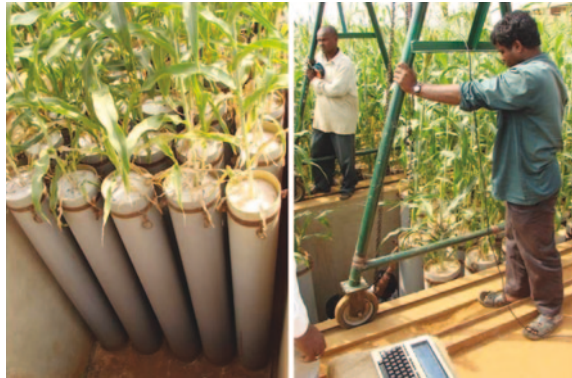
Fig. 13.5 Rhizotronic facility with maize genotypes placed outdoors (at ICRISAT, Hyderabad, India) that allows assessing water balance in plants using a crane
