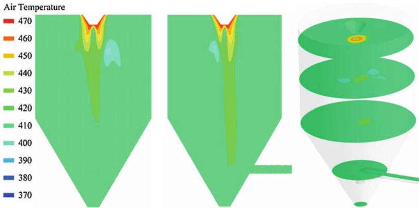
Fig. 4 Flow patterns of air temperature (Kelvin) in spray dryer: frontal ( left ), side ( middle ) and isometric ( right ) cuts
