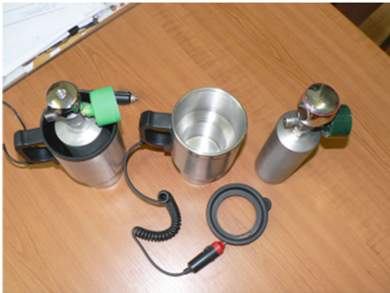
Fig. 16.4 The hydrogen accumulators “Dmisch” supplied with thermostated heat exchangers energized from the constant-current sources of 12 V (see color plates)
