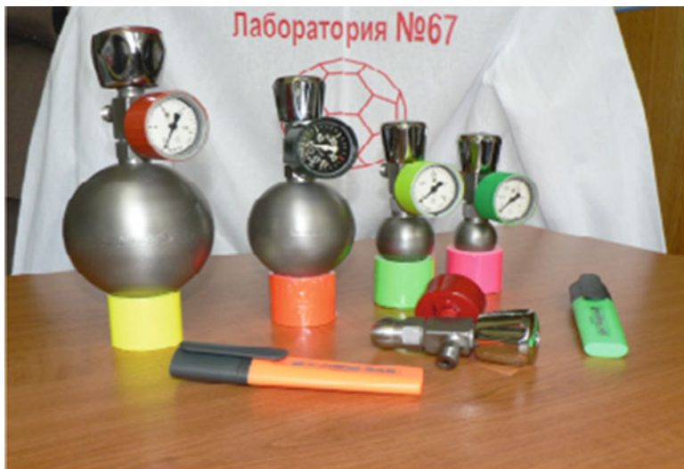
Fig. 16.2 The high-pressure vessels for hydrogen storage and hydrogen accumulators of “Alsav” modification with a capacity of 3, 10, 15, 75 and 170 l
