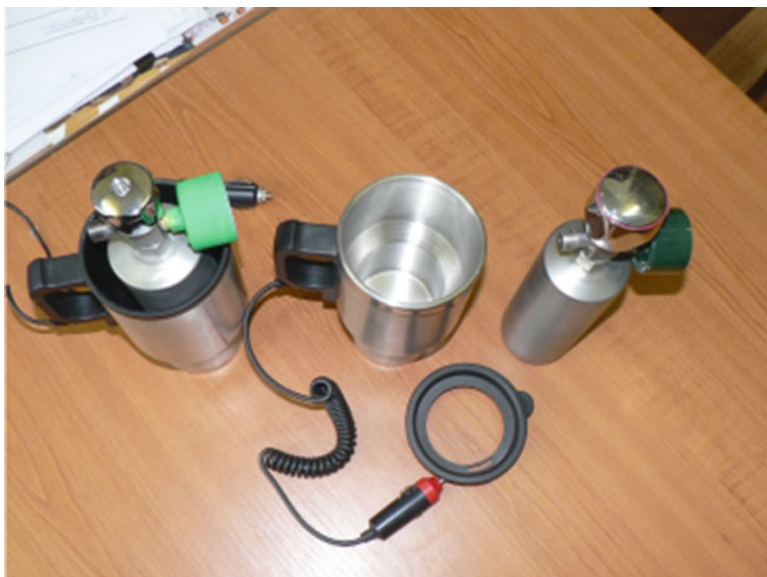
Fig. 16.4 The hydrogen accumulators “Dmisch” supplied with thermostated heat exchangers energized from the constant-current sources of 12 V
