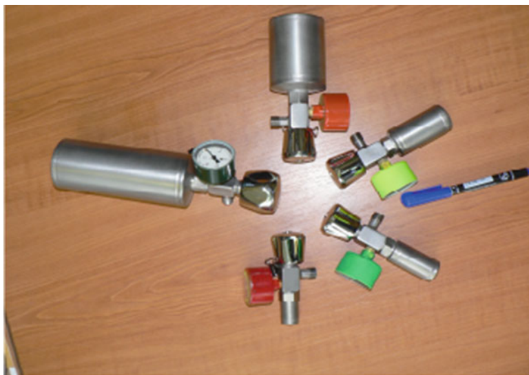
Fig. 16.3 The high-pressure vessels for hydrogen storage and hydrogen accumulators of “Dmisch” modification with a capacity of 3, 10, 15, 75 and 170 l
