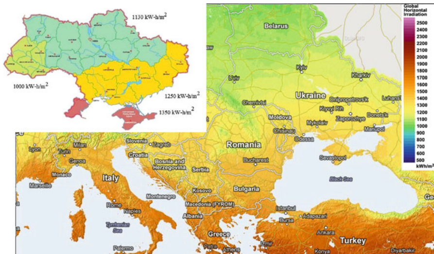
Fig. 10.2 Solar energy potential of Ukraine and neighbouring countries and a more detailed breakdown of the solar energy potential in the regions of Ukraine ( upper left ) (see color plates)
