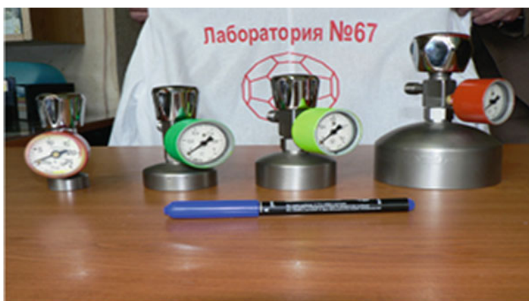
Fig. 16.5 The high-pressure vessels for hydrogen storage and hydrogen accumulators of “Viachbog” modification with a capacity of 3, 10, 15 and 75 l
