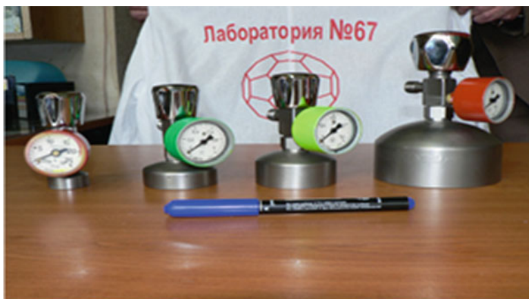
Fig. 16.5 The high-pressure vessels for hydrogen storage and hydrogen accumulators of “Viachbog” modification with a capacity of 3, 10, 15 and 75 l (see color plates)
