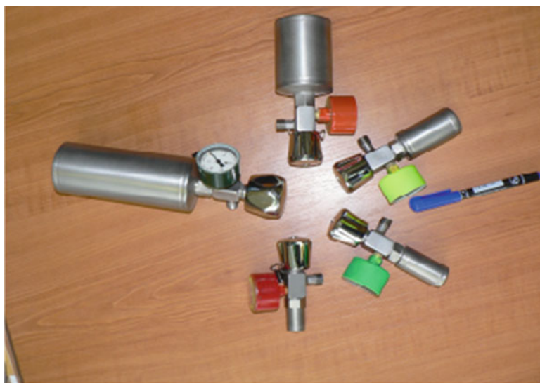
Fig. 16.3 The high-pressure vessels for hydrogen storage and hydrogen accumulators of “Dmisch” modification with a capacity of 3, 10, 15, 75 and 170 l ( see color plates )
