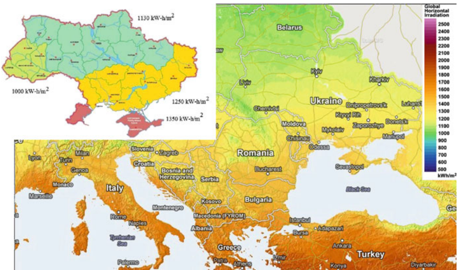
Fig. 10.2 Solar energy potential of Ukraine and neighbouring countries and a more detailed breakdown of the solar energy potential in the regions of Ukraine (upper left)
