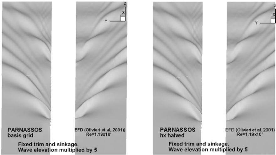
Fig. 3 Comparison between the computed and measured wave elevation for the M5415. Left: computed on the base grid. Right: computed on the base grid after halving the cell size in streamwise direction
