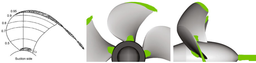
Fig. 5 Euler-Euler simulations of PPTC propeller (Case 1), employing 4 \cdot 10^6 control volumes. Experimentally observed cavitation pattern ( left ), snapshot of predicted vapor volume fraction ( \alpha = 0.2 , centre , right )
