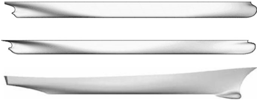
Fig. 1 The three ships used in the workshop (upper: KVLCC2; middle: KCS; bottom: 5415)
