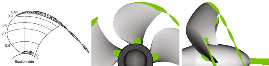
Fig. 6 Euler-Euler simulations of the PPTC propeller (Case 1) employing 12 \cdot 10^6 control volumes. Experimentally observed cavitation pattern ( left ), snapshot of predicted vapor volume fraction ( \alpha = 0.2 , centre , right )
