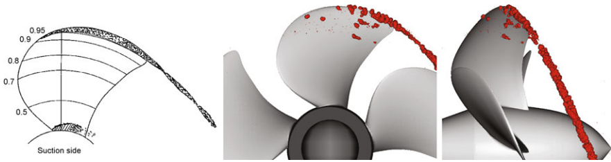
Fig. 12 Application of the Euler-Lagrange model to the PPTC propeller (Case 1) employing 12 \cdot 10^6 control volumes. Experimentally observed cavitation pattern ( left ) and snapshot of computed vapor bubbles ( centre, right )
