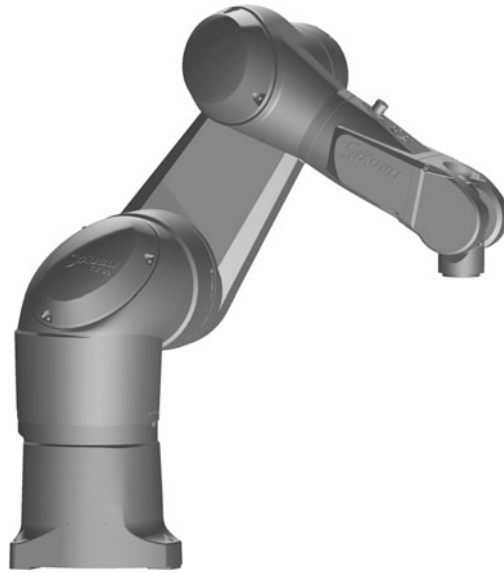
Fig. 5.1 Anthropomorphic Staubli robot
