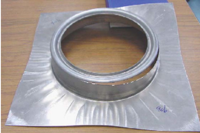
Fig. 6.3 A stretch flange sample fractured by circumferential cracking (Reprinted with permission from Chen et al. (2005). Copyright: Elsevier)
