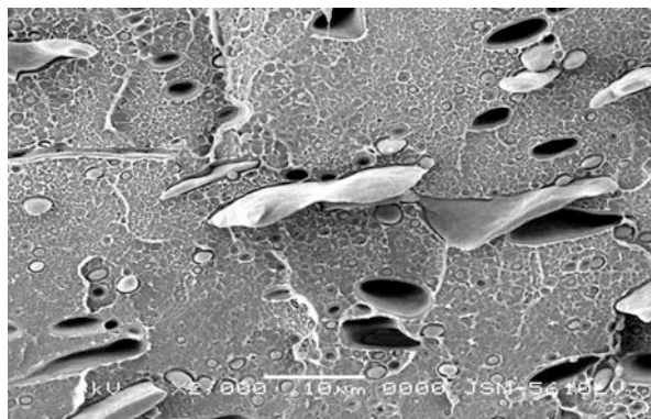
Fig. 10.65 HDPE–polyamide-6 (20 wt%) blend. Injection-molded flexural bar in the skin zone as viewed under SEM (Xavier and Pendyala 2008)
