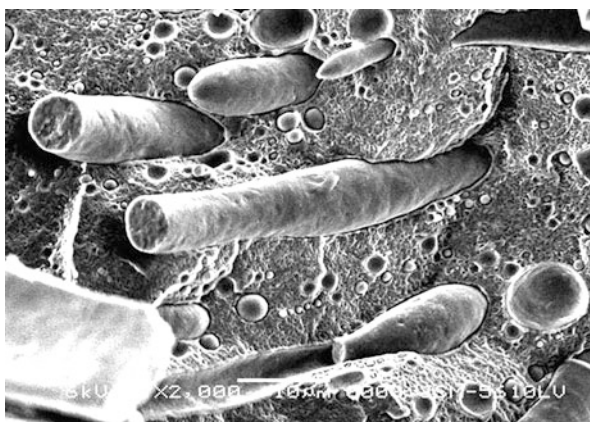
Fig. 10.68 HDPE–polyamide-66 (30 wt%) blend. Injection-molded flexural bar in the core zone as viewed under SEM (Joshi et al. 2005)
