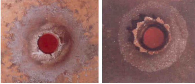
Fig. 13. (a) Front and (b) rear crater damages in Mild Steel plate [16]
