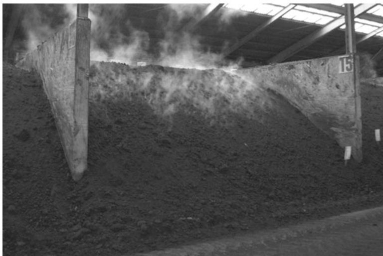
Fig. 4.2 An example of high-temperature compost pile
