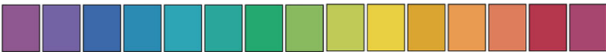
Fig. 13.15 The 15 saturated test color samples used in the CQS (color is not shown in printed version)
