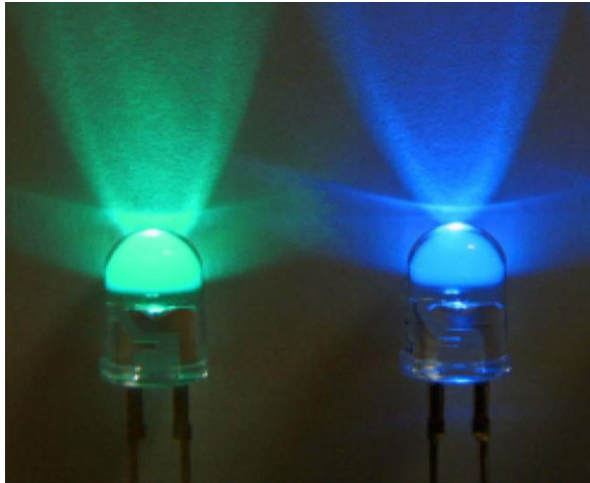
Fig. 3.14 Photographs of the blue and green LEDs on Si emitting at 478 nm and 505 nm (reprinted from Ref. [71] with permission, copyright 2002 Japan Society of Applied Physics)
