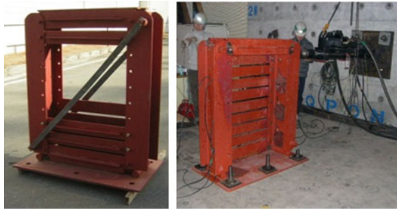
Fig. 5 Shear deformation experiments of SFRW a Steel frame b Horizontal Loading
