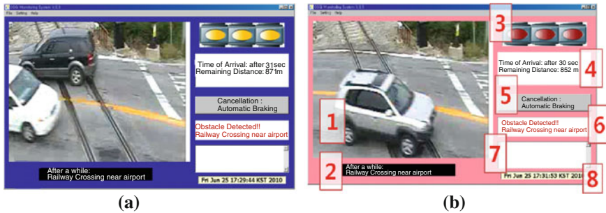
Fig. 6 Monitoring System on Train. a Before crossing barrier was lowered, b after crossing barrier was lowered
