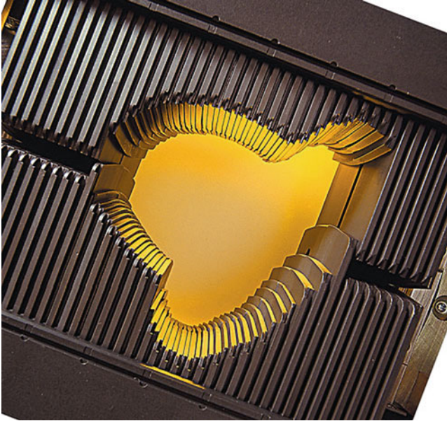
Fig. 20.2 Multi leaf collimator (MLC) is used for sculpting the radiation beam to conform to the shape of the tumor
