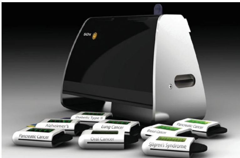
Fig. 34.3 The UCLA Oral Fluid NanoSensor Test (OFNASET) POC device is an electrochemical platform integrated sensitive and specific multiplexing assay, sample collection, sample procession for proteomic and transcriptomic biomarkers in saliva
