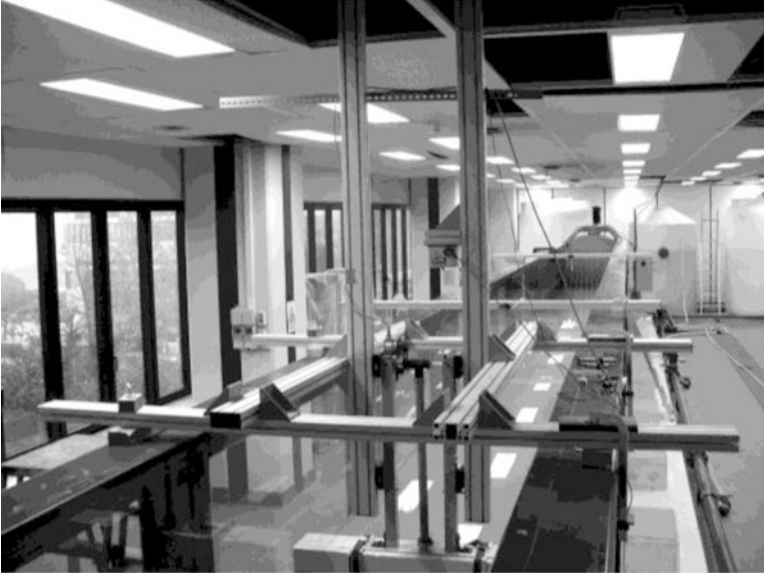
Fig. 2 Photograph showing the Ancona experimental setup where the pendulum system shown in Fig. 3 below is excited by waves generated in a water tank
