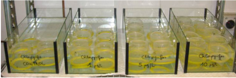
Rapid Tests for Community-Level Risk Assessments in Ecotoxicology, Fig. 1 A typical setup of a rapid test. Each tank contains a different treatment, in which there are baskets that house multiple species in the same test solution but prevent them from physically interacting. In this case, up to eight baskets can be placed in each tank (Photo taken by Alizée Rouane)
