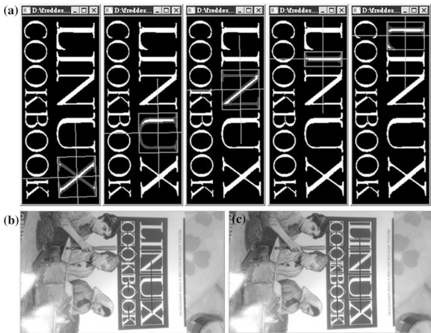
Fig. 2 Example of text-line construction: a directions of text-line seeking with each CC, b connected active components, c constructed text-lines after extension
