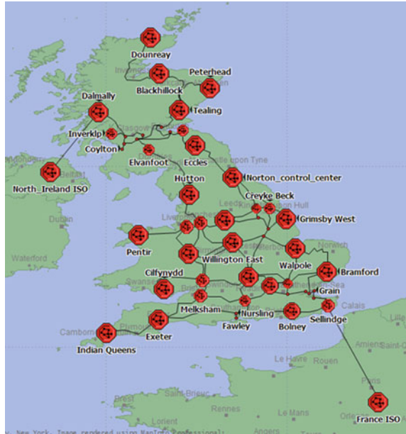
Fig. 2 PMU deployments in United Kingdom according to an optimization based on ILP
