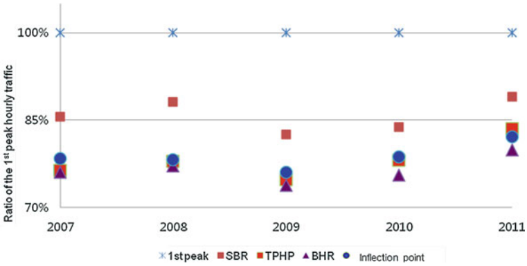
Fig. 4 Comparing ratios of the highest peak hour and design peak hourly traffic
