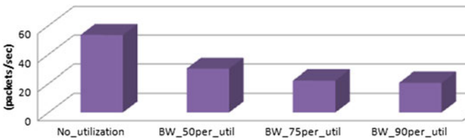
Fig. 15 Point to point throughput of Ulsan to Yeosu for various bandwidth utilizations
