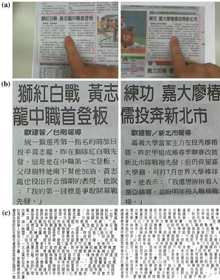
Fig. 8 Two examples of the results of the proposed AR platform. a The result of AC module. b The result of AE module with enlarged ratio of two. c The result of OCR module
