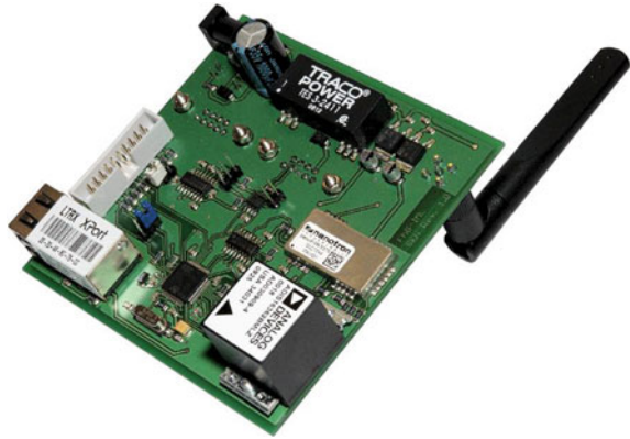
Fig. 4 Wireless sensor node for anchors and mobile tags
