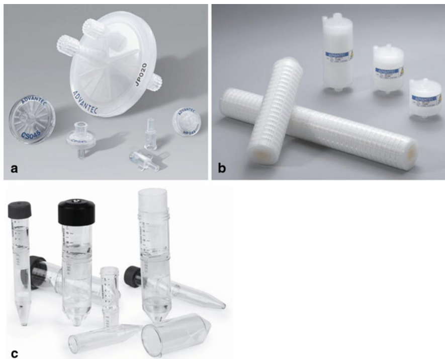
Fig. 4.6 Examples of disposable filtration devices that are available in various sizes and used for relatively smaller sample volumes, ranging from less than 1 ml up to 70 ml, such as a ) syringe filters, b ) capsule cartridges (both photographs provided courtesy of Advantec MFS, Inc.), and c ) centrifugal filtration units (photograph provided courtesy of Sartorius Laboratory Products & Services)
