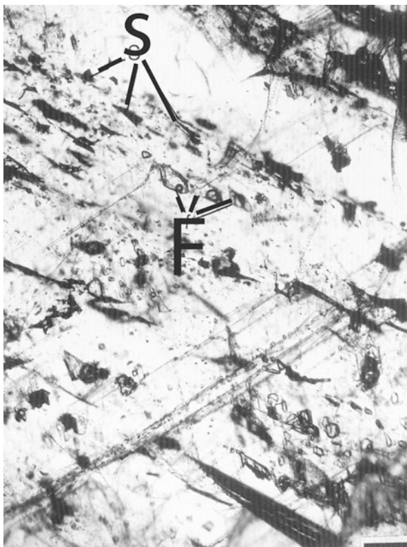
Fig. 5.12 Photomicrograph of fluid inclusions in gypsum crystal, Middle Miocene (~11–16 million years old), Gulf of Suez, Egypt. Solid (S) and fluid inclusions (F, with liquid water and vapor bubbles) occur in planes parallel to the growth direction of the gypsum crystal. Vapor bubbles, not present in original samples, were produced in the laboratory after freezing and melting experiments. Scale bar is 60 \mu\text{m} . (Modified from Attia et al. (1995))
